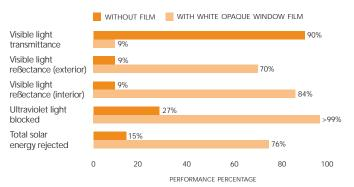
All performance results are based on the  $\hbox{PIm}$  installed on the inside surface of 4mm and 4mm+4mm thick, clear glass.
